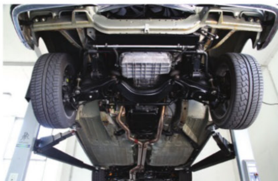
△ Driveshaft from 220 S-Class needed to be shortened.
