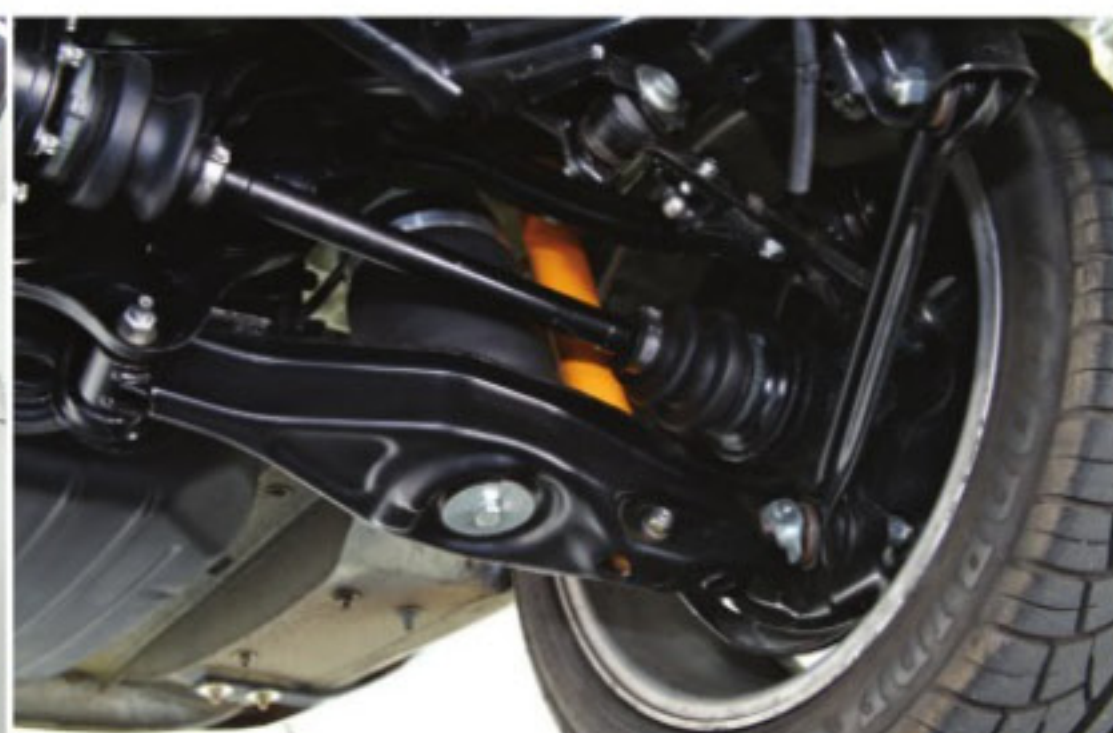
△ Rear S-Class air suspension and Koni dampers all round.
