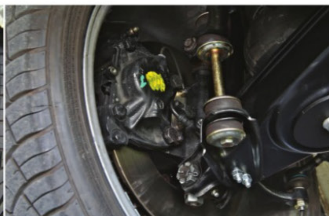
△ Front axle given Firestone's air ride suspension system.
