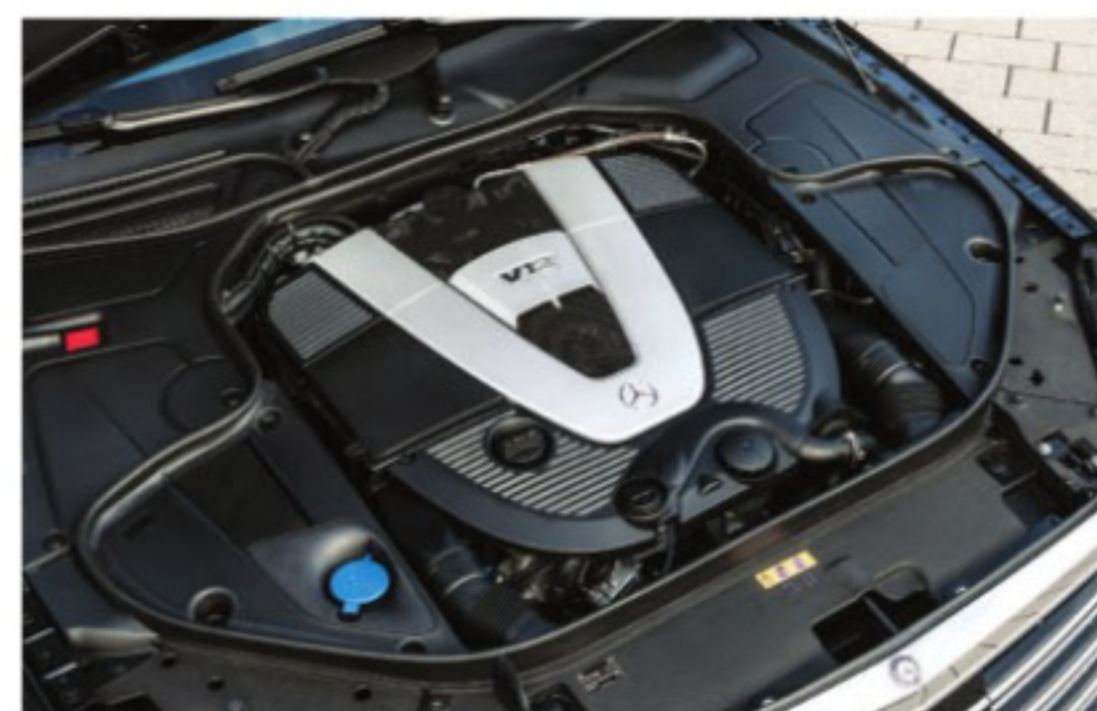
△ The M275 V12 biturbo produces 523bhp/612lb ft torque.
